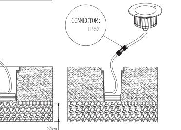
Install the mounting sleeves on the ground , the top side should be on the same level with the ground surface , power cable need to go through the mounting sleeve. Connect the power cable with the lighting fixture. \*keep enough length for maintain\*
