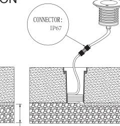
Install the mounting sleeves on the ground, the top side should be on the same level with the ground surface, power cable need to go through the mounting sleeve.
