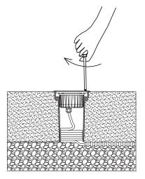
Fix the lighting fixture with the mounting sleeve by a screwdriver.
