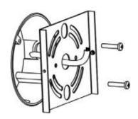
2.Fix the quick installation plate to wall.
