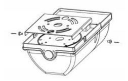
1. Loose screws to take the quick installation plate apart.
