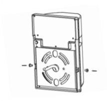
4.Install the fixture body to quick installation plate and tight the screws.
