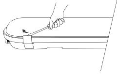
4. Loosen the cable gland and insert the power cable through the cable gland. Select the required wattage & CCT via Switch
