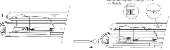
5. Connect the power cable to the driver and tighten the cable gland.
