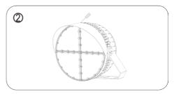
Please use 5pcs M4\*8 screws to install the shading board on the fixture.
