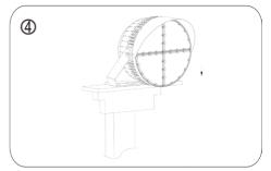
Please loosen the screws on the both sides of fixture, adjust the beam angle of fixture. (Please do not loosen the screws totally)
