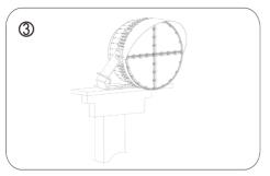
Please install the fixture onto the pole, fasten the screws.
