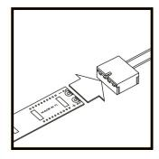
4 You can also connect strips using LED tape connectors.
