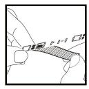
Remove the adhesive tape from the back side of the LED tape.
