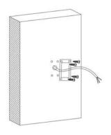
Fix the back cover of the bracket on the wall with two steel screw. Make sure the cable get through the hole in the middle of it.
