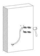
Drill two holes on the wall where you are about to install the lighting fixture. Then put two rubber plug into the holes respectively by using a hammer.
