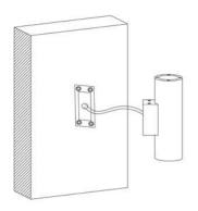
Connect the lighting fixture with the cable which is been prepared for the installation previously.
