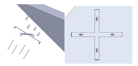
5. Use 4 pcs M4\*20 Screw to fix ceiling disk and Support Bracket from the side. See pictures below for your reference:
