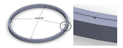
3. Lock the strain relief with M5 hanging pins, see pictures below:
