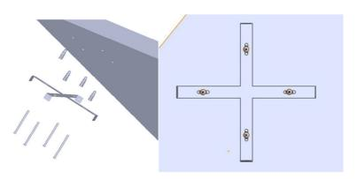
2. Use 4 pcs M54\*20 Screw to fix ceiling disk and Support Bracket from the
