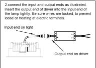
3.Connect wires of driver, directly connect brown and blue input wires to electric supply (220-240V), as shown in the figure:
