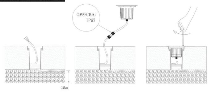
Install the mounting sleeves on the ground, the top side should be on the same level with the ground surface, power cable need to go through the mounting sleeve. Connect the power cable with the lighting fixture. \*keep enough length for maintain\*
